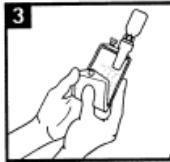
With vial positioned above container, as shown, fold container a third from top and squeeze firmly to transfer solution from vial to container. If necessary, repeat Steps 2 and 3.
